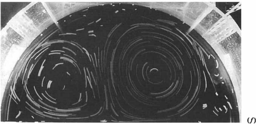
FIGURE 10. Sequence of streakline photographs showing the evolution of the relative flow during the spin-up in the semicircle geometry, taken at (a) t = 0.4T , (b) 1.0T , (c) 1.8T , (d) 2.4T , (e) 5.4T , and (f) 14.4T , with T = 8.3 s the rotation period. The exposure time of (a–e) was 1 s, whereas the exposure time of (f) measured 3 s. Experimental parameters: H = 12.5 cm, \Omega = 0.756 rad/s.
